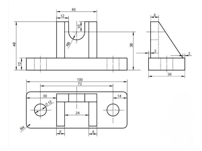
3) Draw the isometric view of the part in which three different views of it are given in the below.(30 pts)
