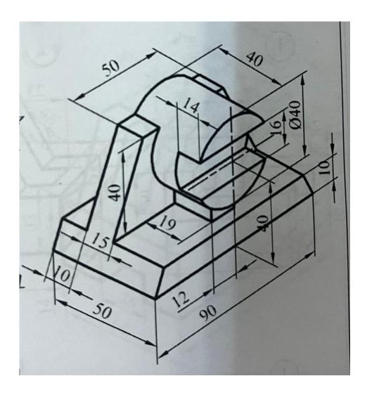
2) Draw front, left and side views of the part shown below and make dimensioning.(30 pts)
