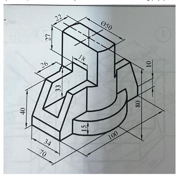
3) Draw the isometric view of the part in which three different views of it are given in the below. (30 pts)
