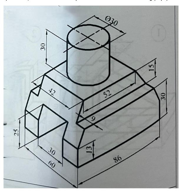
3) Draw the isometric view of the part in which three different views of it are given in the below. (30 pts)
