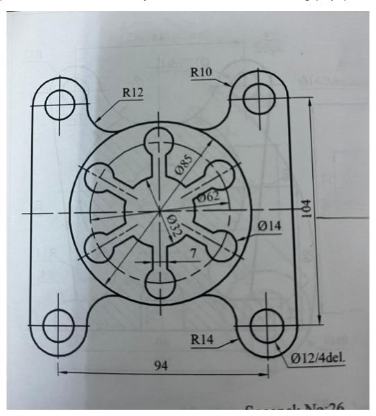
2) Draw front, left and side views of the part shown below and make dimensioning. (30 pts)
