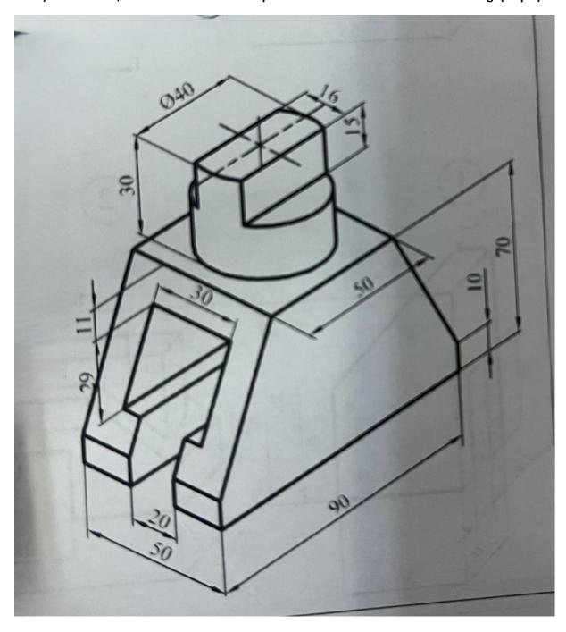
3) Draw the isometric view of the part in which three different views of it are given in the below. (30 pts)
